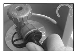
Check the bullnose connection on the regulator for any visible damage before connecting to the cylinder.
