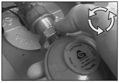
Tighten firmly using a gas spanner (or an adjustable spanner), continuing in an anti-clockwise direction.
